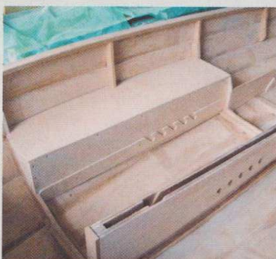
22 The side benches double up as buoyancy aids, with the slots for the forward foot braces on either side (the slots haven't been fitted to the centreboard case yet).
