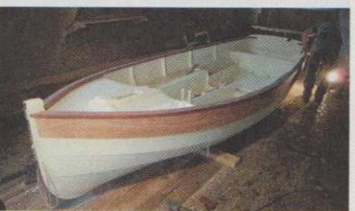
25 Et voila! The hard work pays off as painting is completed and the sheerstrake receives coats of varnish.
