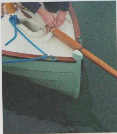
A couple of lashings are all that's required to hold the sprit in place
