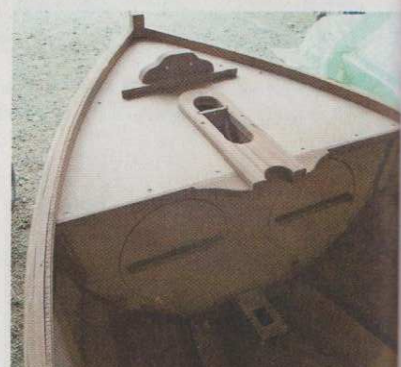
23 The forward deck is fitted, with the mast partner in place. The box for the forward mast step (for the cat rig) passes through the forward compartment, accessed through the round hatches.
