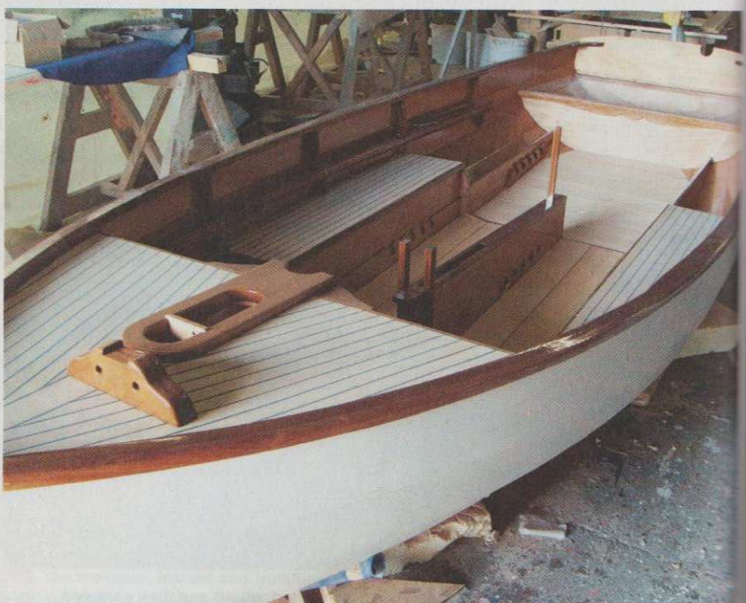
26 This is the deluxe version fitted with a veneered deck, varnished Columbia pine floor boards and a clear finish to the interior woodwork.
