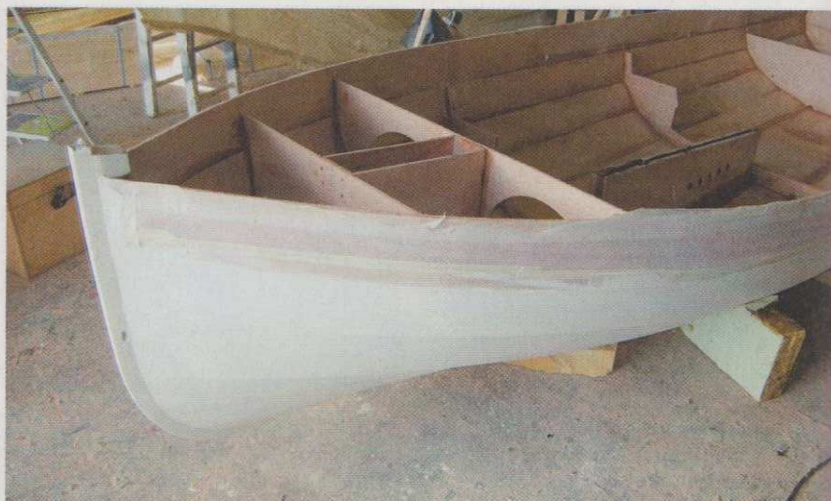
20 The shearstrakes of this boat have been cleverly masked off to prevent them being painted over. Once the lower strakes are painted, the covering was removed and the shearstrake varnished.
