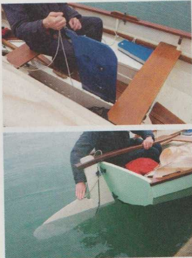
Centreboard/daggerboard and tiller are held in place by simple notches and pins
