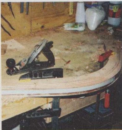
4 The inner stem is made from several layers of ply epoxied together and bevelled to take the hood ends. No need for a complicated laminating jig.
